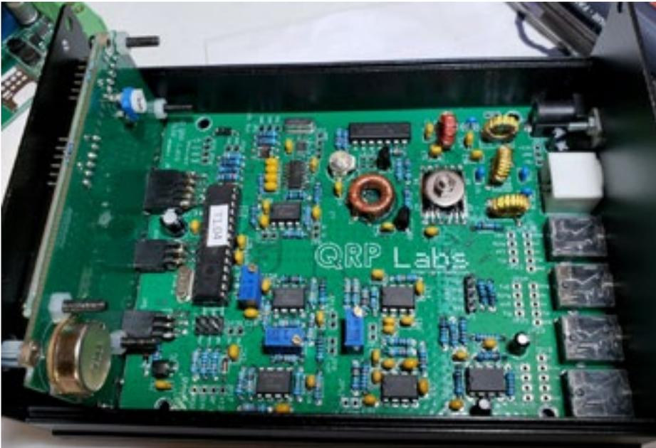
of these include: a built in iambic keyer, pre-stored messages, a CW decoder and more. All of these can be controlled via a set of pushbuttons and a rotary encoder and displayed on a 16x2 LCD panel. The whole rig can be run for many hours from a 12V 12000mAh Li-ion cell pack which makes it a great rig for a QRP “expedition” to a local park.
