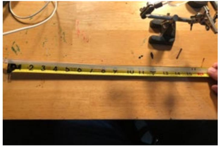
Lets go back to the table and lay out the antenna flat again. You will need to measure 15.25 inches from where you just nibbled and tinned the twinlead wire. At this mark cut a .25-inch notch into ONLY ONE SIDE of the twinlead.
