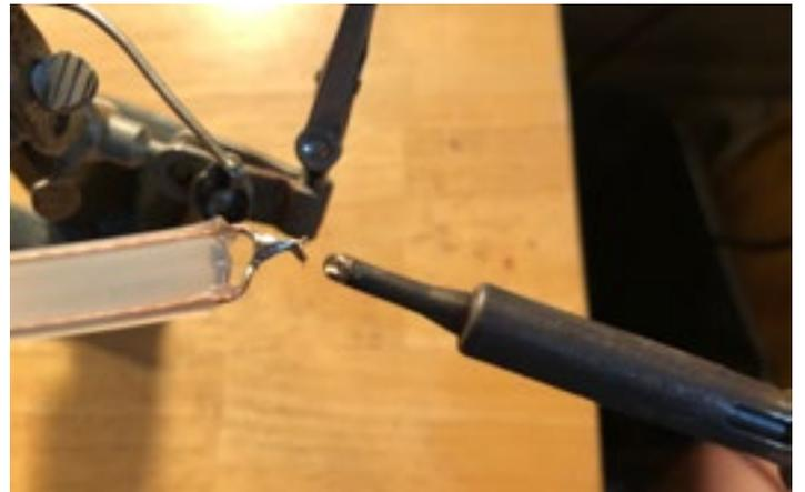
(While holding the correct end of the soldering iron.....Sorry poor Internet joke that has been around) Use the soldering iron to heat up the twisted wires and apply some solder and it should flow right on to the wires. Let it cool down for a minute and you can clip off the excess wire that is not needed.
