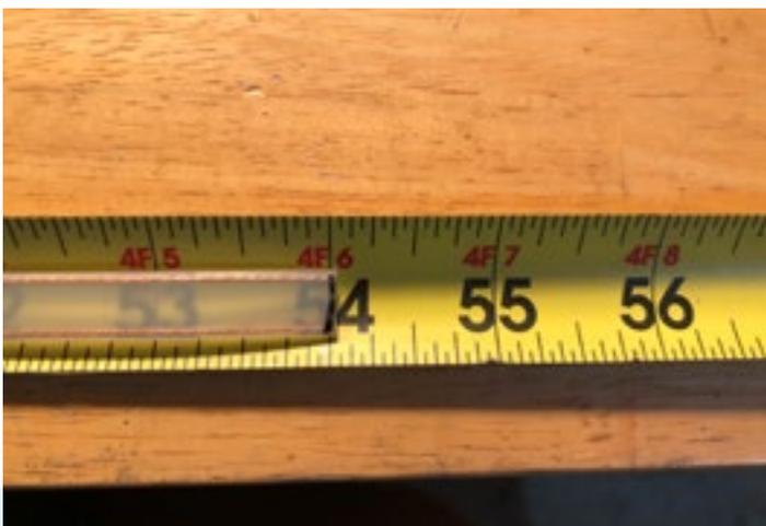
Lets make the last cut that we need to do on the twinlead. Place the twinlead back on the table and from the bottom of the antenna, where we twisted and soldered the two wires, measure up 54 inches and CUT. This is now the length of the antenna. Do not put that soldering iron away yet the most important connection is coming up. So, clean the tip of it and put it in its holder.
