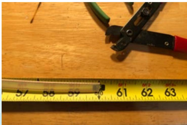
Following the instructions on the website, the first thing to do is cut a section of the TV twinlead to 60 inches long. I laid it out flat on the table and gave it a snip at the 60" mark.
