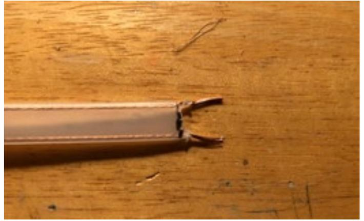
Once that it done pick one of the ends and draw a line on the cable ½ inch up. This will be the bottom of the antenna. Remove the insulation around the wires, trying not to cut the wires. You can take the two wires and twist them together. Now warm up that soldering iron.
