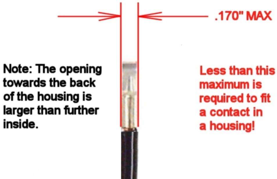
**YOU WILL NOT BE ABLE TO INSERT THE CONTACTS INTO THE HOUSINGS IF THEY ARE TOO WIDE AFTER SOLDERING OR CRIMPING!**
