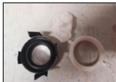
Here is the front cover from the Shure 444. The four pieces of tape are used to secure this cover to the PVC fitting that screws on the front of my boom mike. I later wrapped tape around the joint to better secure the cover.
