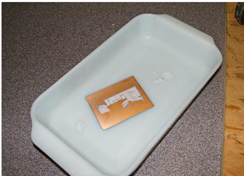
Figure 8. Most of the paper has been removed. Scrubbing with your fingers under running water will remove the rest.
