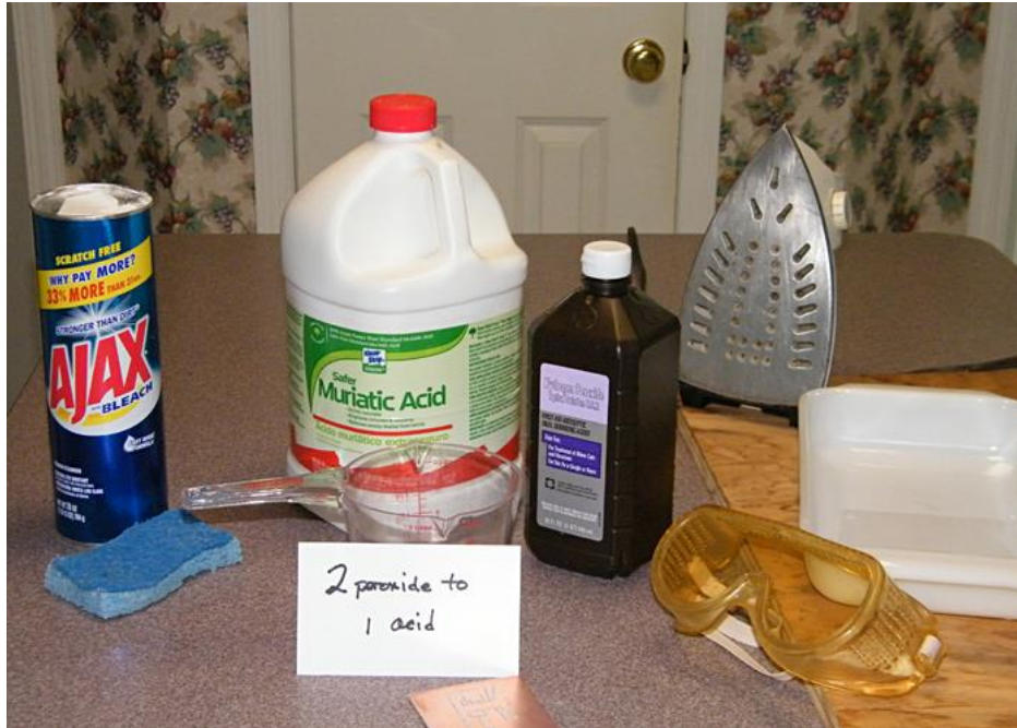
Figure 10. Notice I have a plastic measuring cup, and a glass tray for processing. Do not use aluminum, or other metal pan for etching. Use only glass or plastic.
