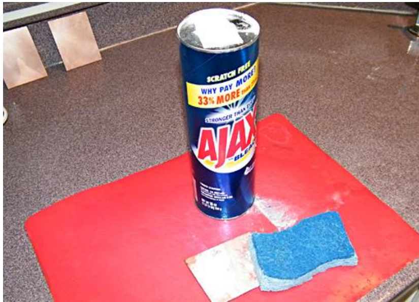
Figure 4. Cleanser is a good choice for cleaning the copper on the board.
