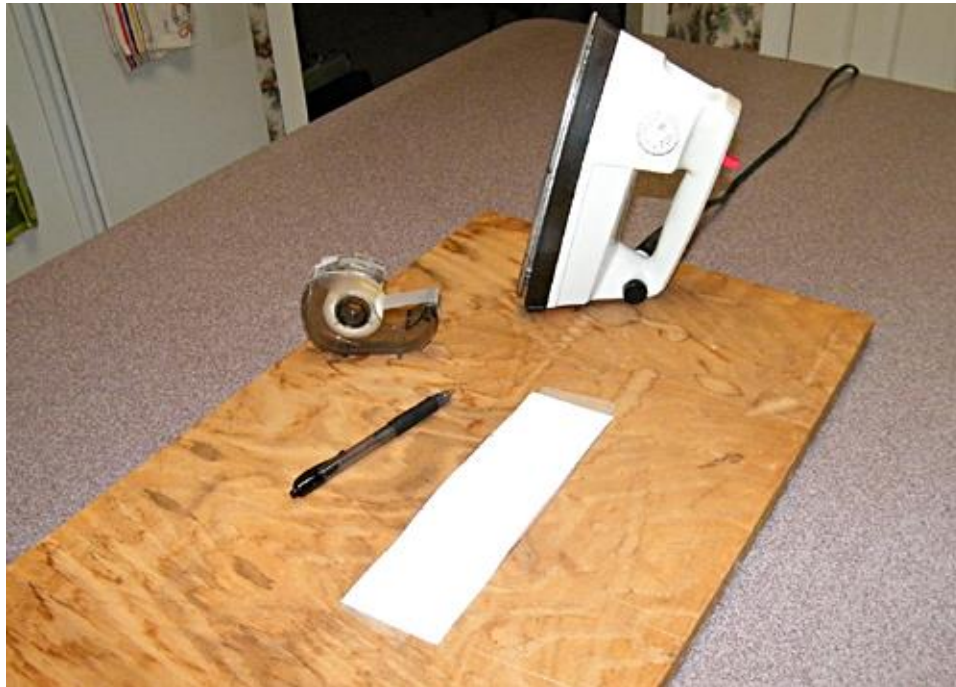
Figure 6. The board is affixed to the work surface and under the sheet of paper containing the circuit. The image is face down.
