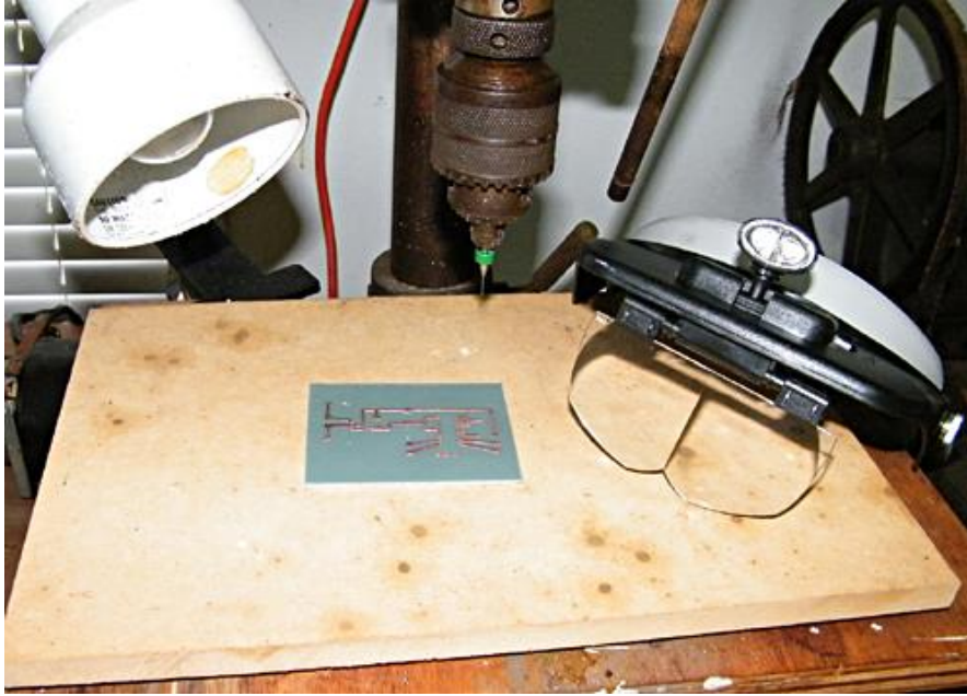
Figure 16. Board drilling setup
