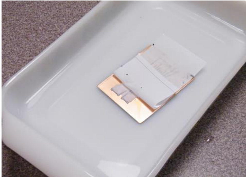
Figure 7. After a minute or so the paper will come away from the board.
