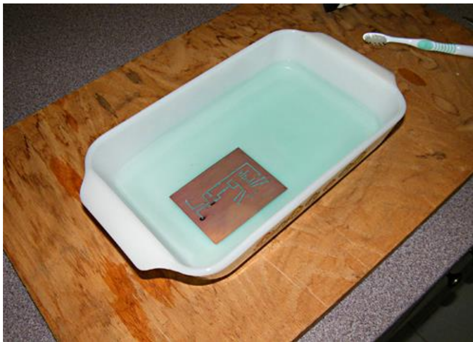
Figure 11. Board first immersed into the etching solution
