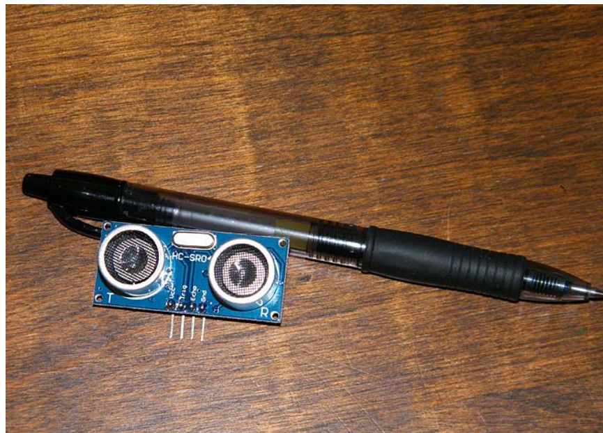
Figure 1. The sensor is relatively small. The left side labeled T is the transmitter; the right, labeled R, is the receiver.
